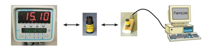
The operating principle of FarmLink is based on the cartridge, movable memory particularly resistant and conceived for severe environments such as the farm. The functions of the cartridge are mainly two: the first one allows to "store" the theoretical data coming from the program by means of a proper interface. The second one allows to record all the operations carried out by the feeder: real consumptions, starting date/time of loadings/unloadings and relevant duration of the operation.
